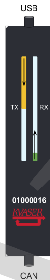
Figure 3: The Tx LED bar lights up from the USB side to the CAN side of the unit, while the Rx LED bar lights up from the CAN side to the USB side of the unit.
