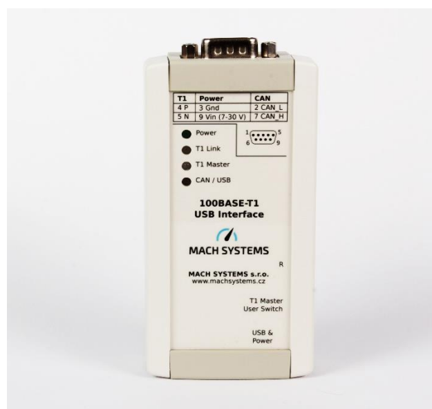
Figure 2 100BASE-T1 USB Interface
