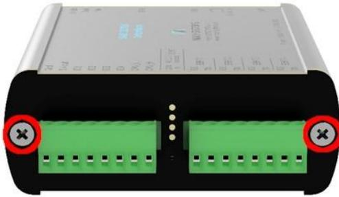
Figure 42: Screw Removal
