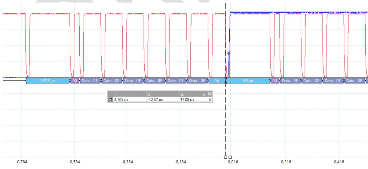
Figure 47: TdSA Measurement Illustration
