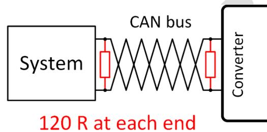
Figure 6: CAN bus termination
