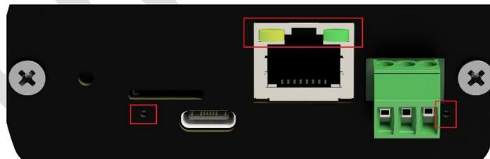
Figure 5: Back Side LEDs
