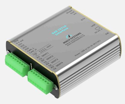
The **SAE J2716 Interface** features four SENT channels, an Ethernet port, a USB port, a CAN(/FD) channel, four analogue channels and a MicroSD card slot. The device can be used as a SENT to Ethernet/USB/CAN(/FD) gateway, a SENT-analogue converter, a stand-alone SENT and CAN(/FD) data logger, or as an Ethernet-CAN(/FD) or a USB-CAN(/FD) interface.
