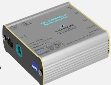
**The 100/1000BASE-T1 Media Converter H-MTD** establishes a point-to-point link between the Automotive Ethernet and Standard Ethernet, supports both 100 Mbit and 1000 Mbit speeds, and features the Rosenberger H-MTD connector.
